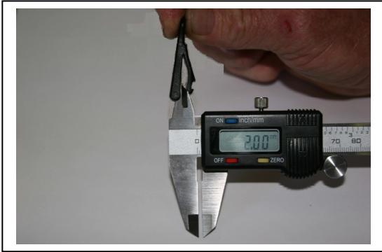
Figure 25 Batten End Fitting Dimension Check
