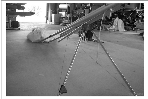
Figure 12 Frame Preparation for Sail Reinstallation
