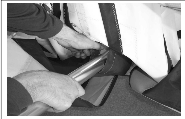
Figure 15 Inserting Keel Into Sail
