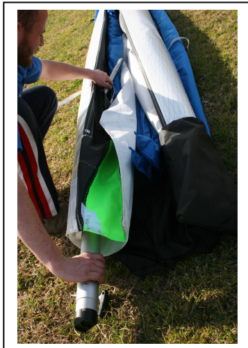
Figure 1 Insertion of Rear Leading Edges
