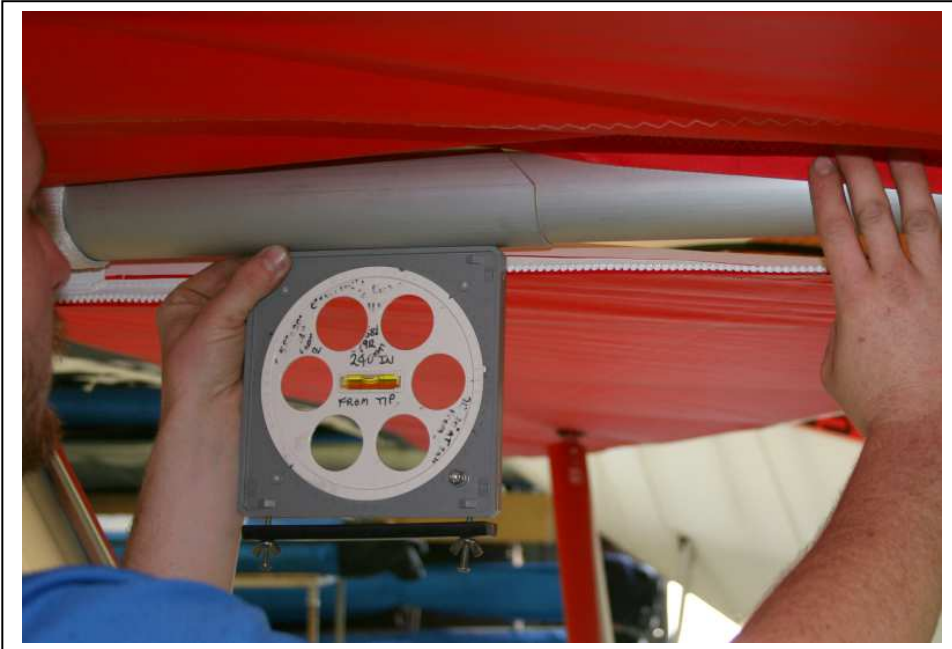
Figure 26 Setting Reference Keel Angle
