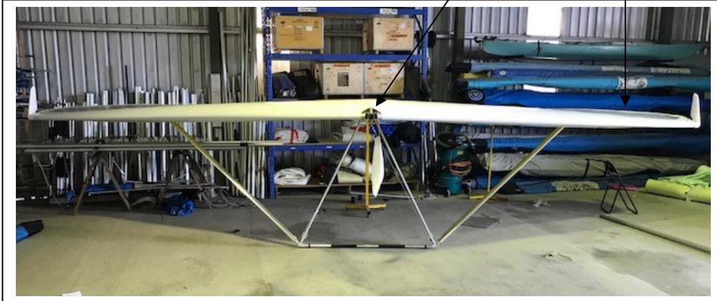
Figure 35 Visual Symmetry Check – Front View
