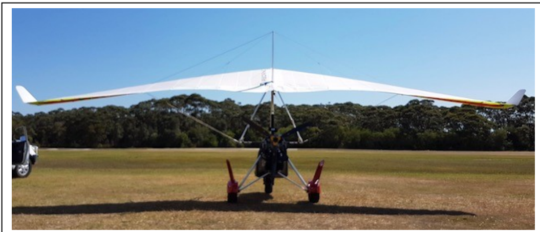
Figure 36 Visual Symmetry Check – Rear View
