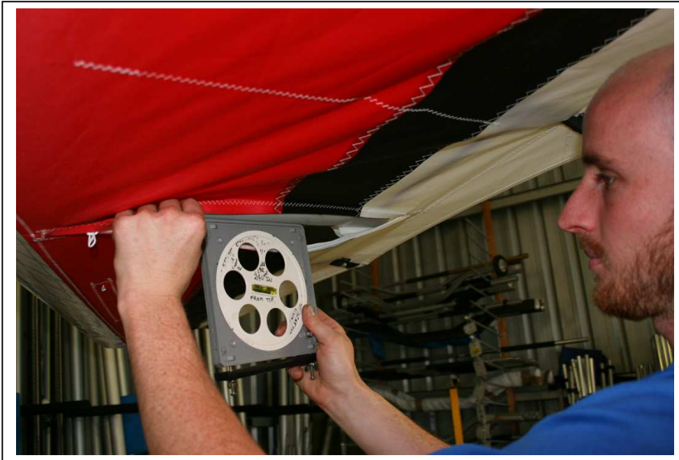
Figure 28 Checking the Outer sprog angle
