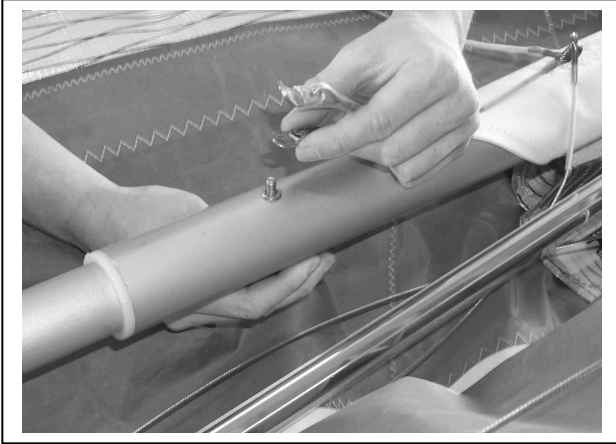
Figure 9 Removing Rear Wires
