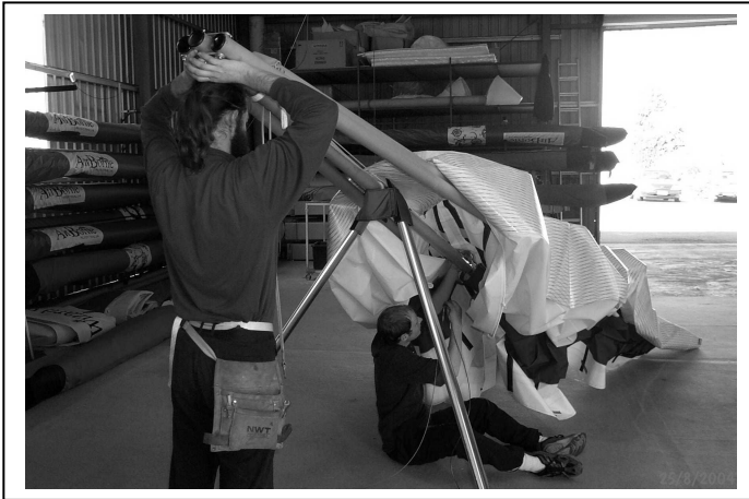
Figure 16 Position Keel Pocket Forward Of Rear Wires
